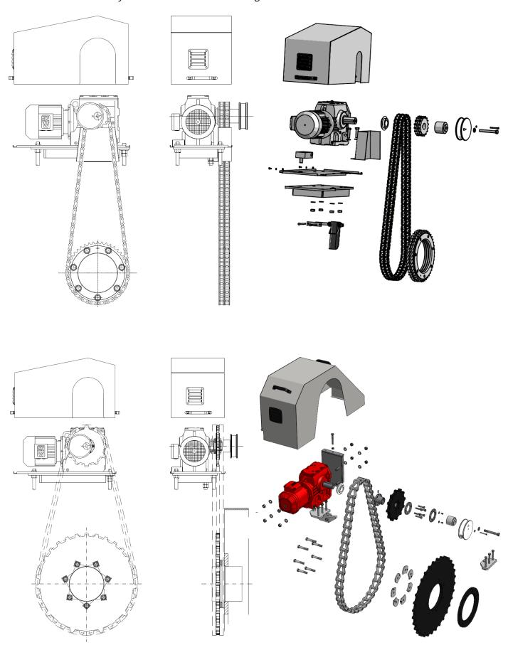
The top image illustrates the old duplex drive assembly and the lower image illustrates the newer H78 narrow chain drive.
