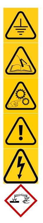
Symbol is displaying equipotential earth bonding points on the filter.
