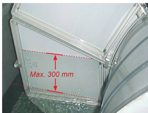
Figure 5.2.2 Maximum allowed differential pressure in AUTO mode
