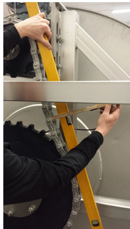
Figure 8.11 Checking drive chain tension
