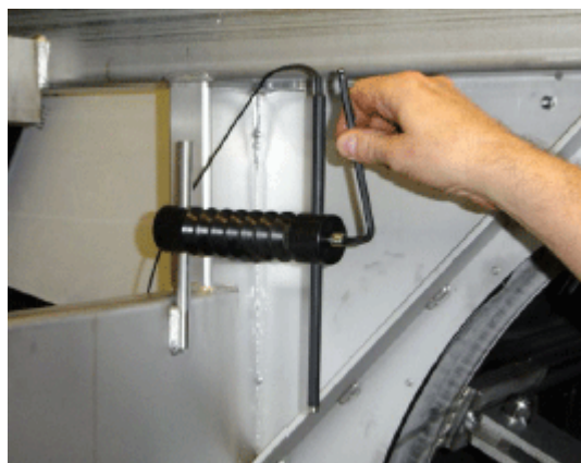
Figure 6.4 Adjusting the level sensor
