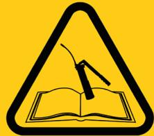
Symbol shown at lubrication points on the filter. Read the manual for further information about lubrication.
