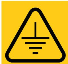
Symbol is displaying equipotential earth bonding points on the filter.
