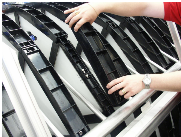
Figure 7.18 The filter segment cover is removed.
