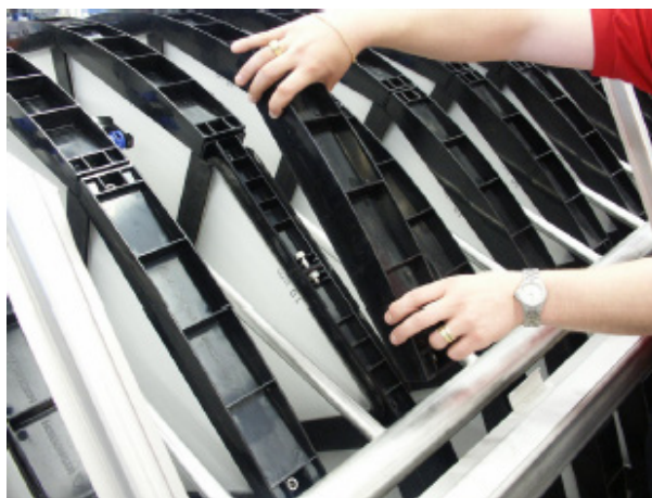
Figur 7.11 Filtersegmentets lock tas bort.
