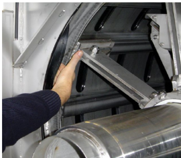
Figure 6.31 Check of inlet seal.
