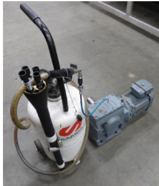
Figure 6.32 Drive unit drained with pump.
