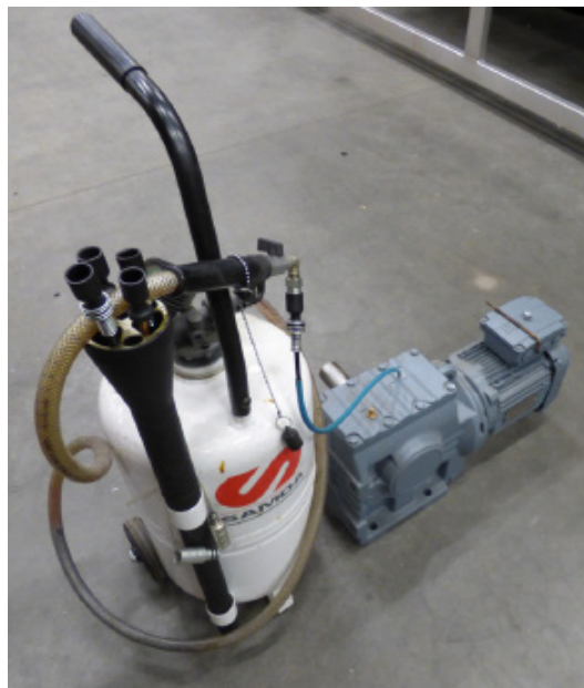
Figur 6.32 Oljan töms ur drivenhet mha pump
