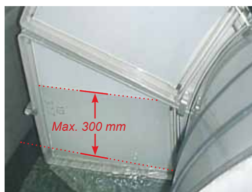
Figure 5.2.2 Maximum allowed differential pressure in AUTO mode
