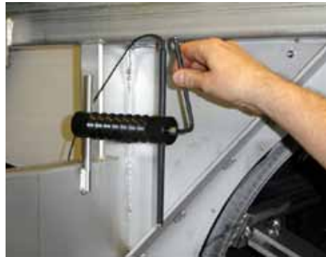
Figure 5.5.2 Adjusting the level sensor
