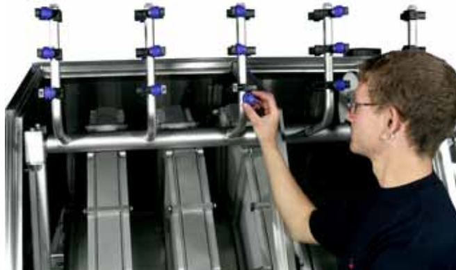
Figure 7.1.1 Spray bar lever lifted and a nozzle removed
