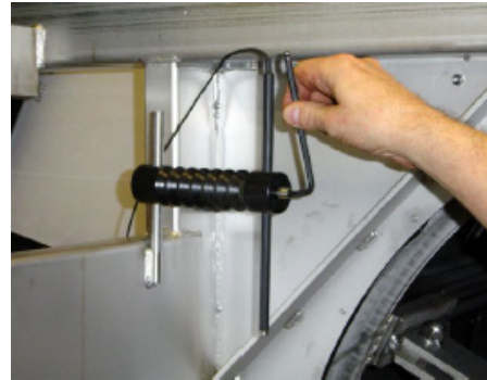
Figure 5.4 Adjusting the level sensor.
