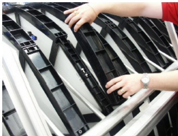
Figure 7.11 The filter segment cover is removed.
