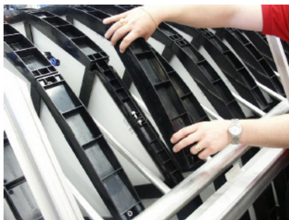
Figur 7.11 Filtersegmentets lock tas bort.
