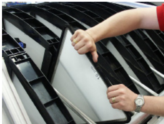
Figur 7.12 Filterpanelen dras ut.
