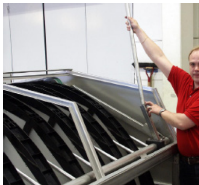
Figure 7.2 a) Place the loose lever in the bracket.
