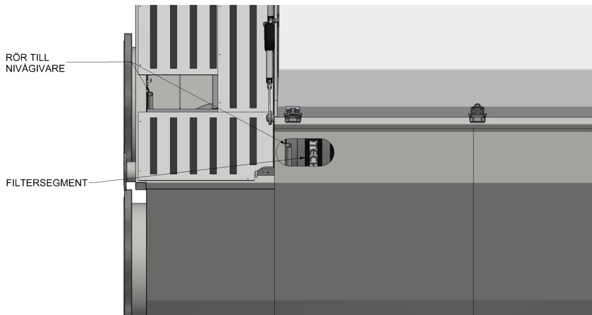
Figure 3.5 Hydrotech Discfilter in HSF2600 series type 1F with a chequered plate removed on the inlet side and a transparent side plate. The level sensor behind the transparent side plate will be available once you lift the cover on the backwash pipe side.
