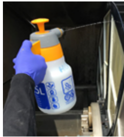
Figure 8. Portable pressure spray bottle used for application of cleaning chemicals on the filter media.
