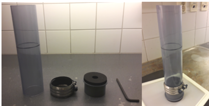
Figure 4. Test tube and insert for measuring long-term fouling of the filter media.
