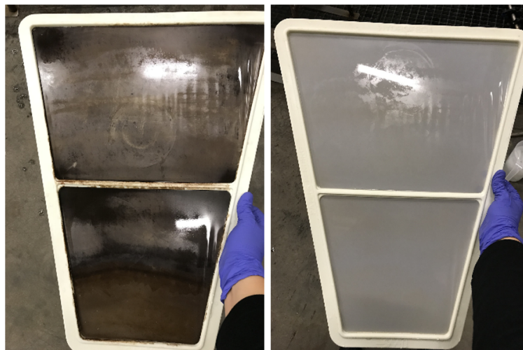
Figure 3. A disc filter panel from an installation with iron based coagulant dosing, before (left) and after (right) chemical cleaning.
