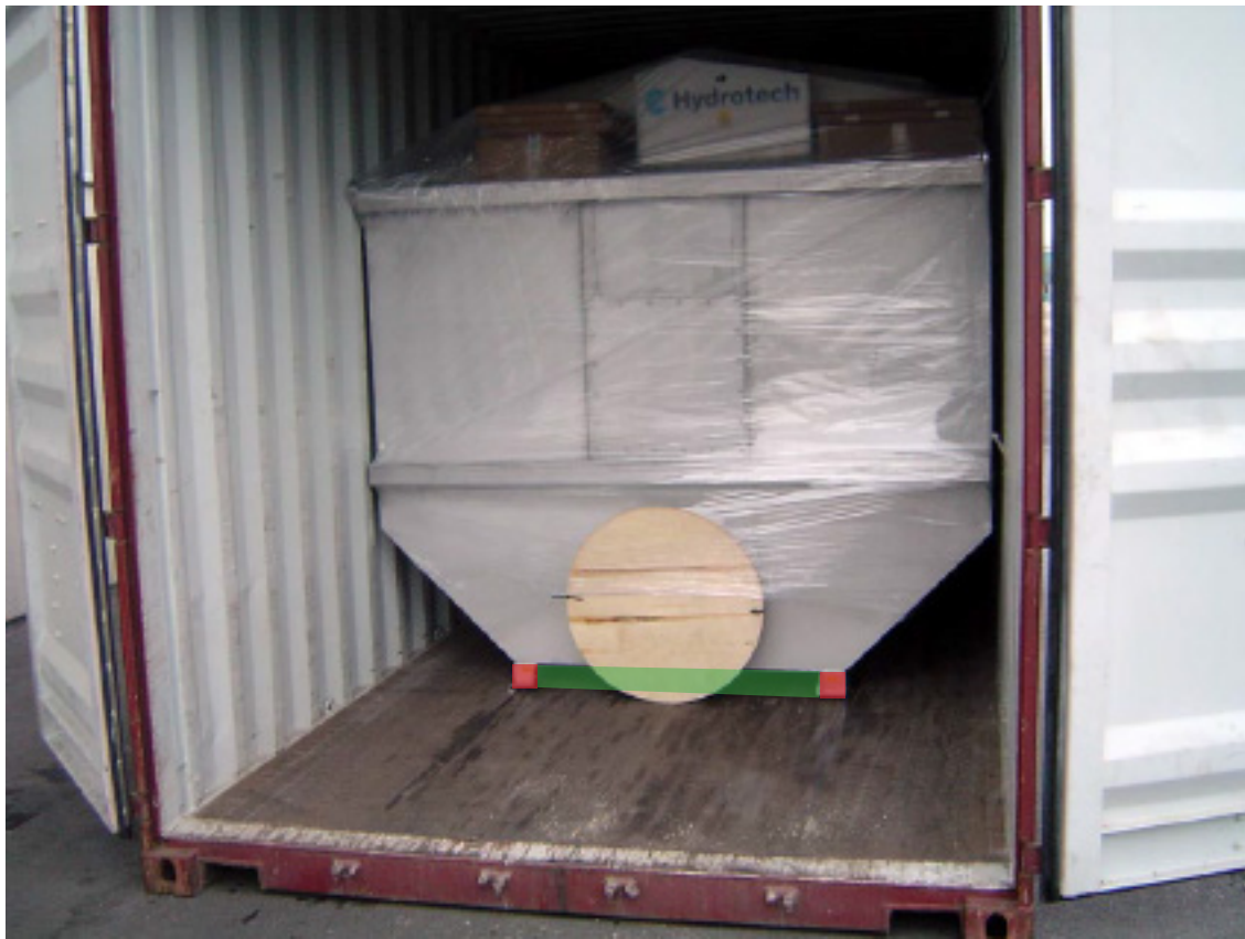
Figure 1, Space for forks marked in green. Chain shackles can be attached on feet marked red.
